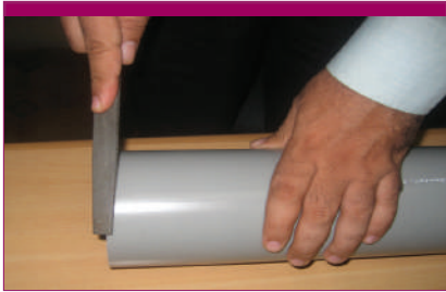
Remove all burrs & chamfer the external pipe edge
