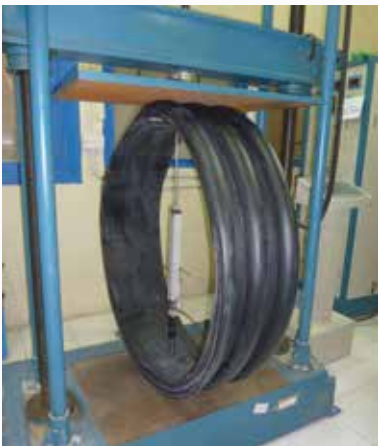
Ring stiffness testing as per ISO 9969
