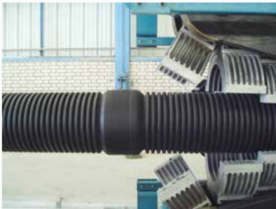
Production of NIC HDPE corrugated pipes with integrated socket
