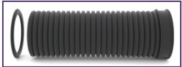
The **pipe** is a high density co- extruded twin wall pipe, smooth internally and externally corrugated with stiffness class SN8 kN/m<sup>2</sup> (on request it is possible the class SN 16 kN/m<sup>2</sup>).
